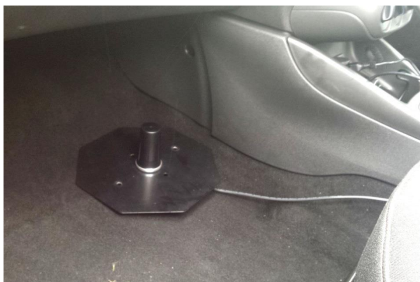
Figure 6: Antenna position in the footwell
