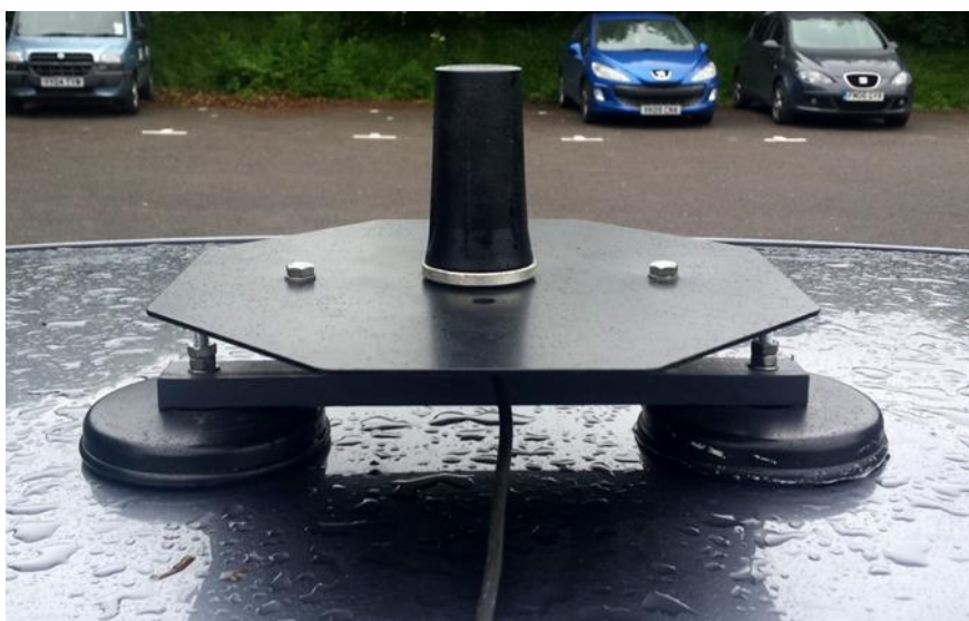
Figure 4: Broadband Test Antenna and Ground Plane
