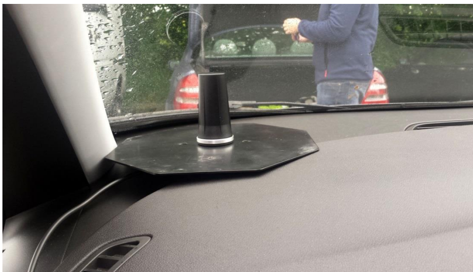
Figure 5: Dash mounted antenna position
